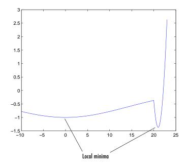
The function has two local minima, one at x = 0, where the function value is - 1, and the other at x = 21, where the function value is - 1 - 1/e. Since the latter value is smaller, the global minimum occurs at x = 21.
