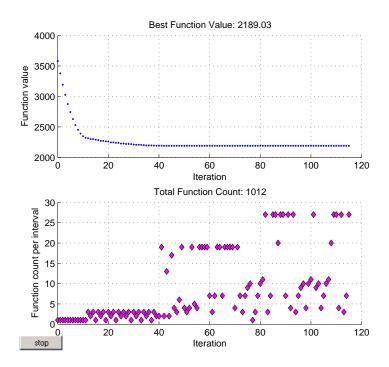
Note that using the search method reduces the total function count — the number of times the objective function was evaluated — by almost 50 percent, and reduces the number of iterations from 270 to 120.
