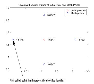
The algorithm polls the mesh points by computing their objective function values until it finds one whose value is smaller than 4.6347, the value at x0. In this case, the first such point it finds is  $[1.1 \ 1.7]$ , at which the value of the objective function is 4.5146, so the poll at iteration 1 is *successful*. The algorithm sets the next point in the sequence equal to
