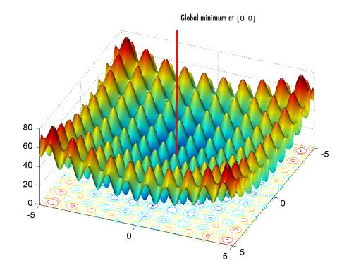
As the plot shows, Rastrigin's function has many local minima — the "valleys" in the plot. However, the function has just one global minimum, which occurs at the point  $[0 \ 0]$  in the *x-y* plane, as indicated by the vertical line in the plot, where the value of the function is 0. At any local minimum other than  $[0 \ 0]$ , the value of Rastrigin's function is greater than 0. The farther the local minimum is from the origin, the larger the value of the function is at that point.
